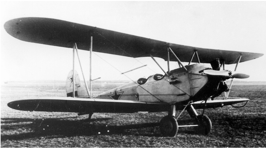
The venerable Polikarpov U-2 (re-designated the Po-2 in 1944) served as the VVS-KA's elementary trainer throughout World War II, some 13,500 examples having been built by June 1941. Praised for its positive longitudinal stability and reluctance to spin, the pedestrian U-2 was the ideal tool for the hundreds of flying clubs charged with training pilots for frontline units.
