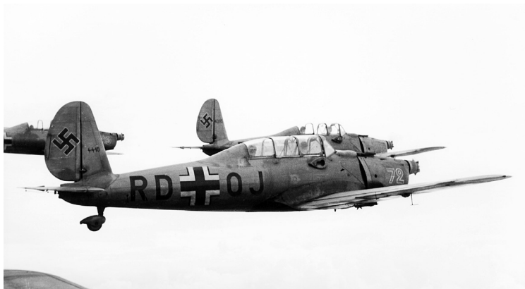
Luftwaffe student pilots practise formation flying in Arado Ar 96A trainers. Used for advanced, night and instrument flying training, the Ar 96 was a single-engine, low-wing monoplane of all-metal construction.
