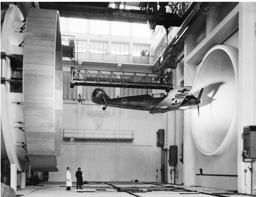
A pre-production Bf 109E undergoes airflow testing in the full-scale wind tunnel at the Luftfahrtforschungsanstalt Hermann Göring Aerial Weapon Establishment , one of the Luftwaffe's leading centres for top-secret development located on the outskirts of Braunschweig. The fighter is suspended on cables rather than mounted on the usual rigid posts.
