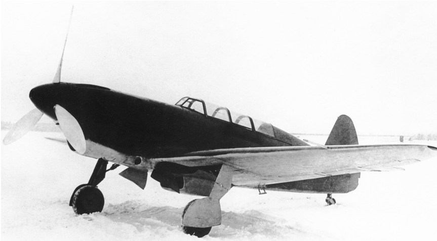
A UTI-26 two-seater in the course of testing in early spring 1941. Note the main undercarriage legs, which differed from those of the Yak-1, the non-retractable tailwheel, the two-seat canopy and the oil cooler channels now moved to the wing roots.
